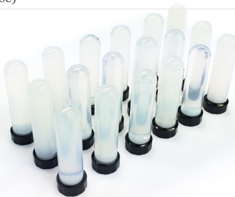
A set of 18 gel-filled tubes with calibrated T1 and T2 values (Available separately).
