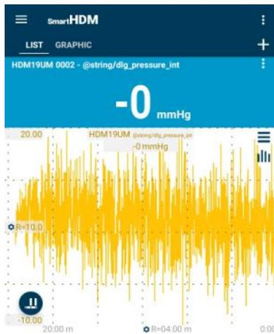
The graph shows that the measured value fluctuates strongly around 0, +/- 20 mmHg.
