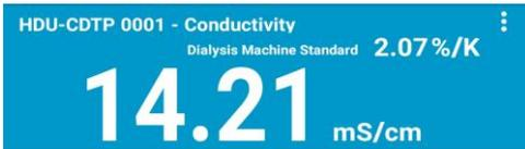
Here “Dialysis Machine Standard” shows the selected conductivity temperature compensation coefficient.
